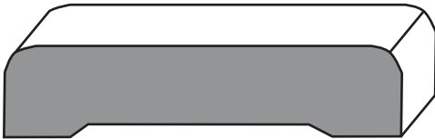
ROUND EDGE MC452 9/16 X 1 5/8 FJP, MC453 9/16 X 2 1/4 FJP, SP, MDF MC433 9/16 X 3 1/4 FJP, SP, MDF MC436 11/16 X 3 1/4 MDF MC434 5/8 X 3 1/2 VG FIR CS003 3/4 X 4 1/4 FJP
